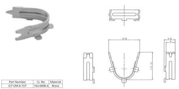
Note: This terminal suits cables having an outside diameter of 8.6 to 8.8 mm.
